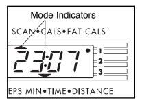
a flashing mode indicator will show which mode is currently displayed. Note: If you select a different mode, you can select the scan mode again by repeatedly pressing the mode button.
